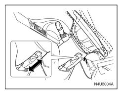
The lever that allows you to tilt the steering wheel is located under the steering column.
